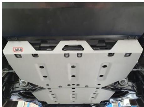
**KIT BLINDAGE DE PROTECTION RADIATEUR MOTEUR DIFFÉRENTIEL AVANT ARB 3 MM POUR TOYOTA LAND CRUISER J250**
