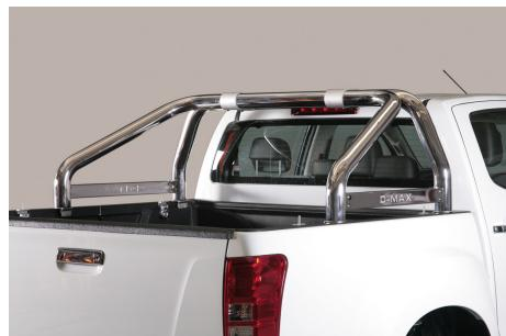
**ROLL BAR INOX DOUBLE TUBE Ø 76MM POUR ISUZU D-MAX A PARTIR DE 2012**
