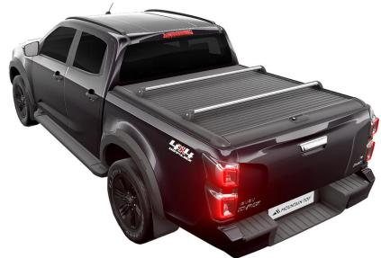
**BARRES DE PORTAGE POUR COUVRE BENNE
