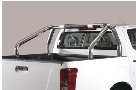
**ROLL BAR INOX DOUBLE TUBE Ø 76MM POUR
