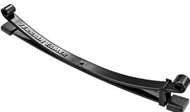
**LAMES PARABOLIQUES ARRIERE TERRAIN
