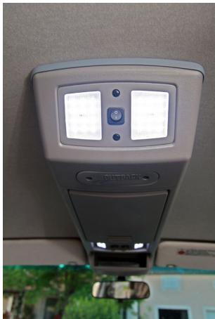
**CONSOLE DE TOIT LONGITUDINALE ARB POUR ISUZU D-MAX DOUBLE CABINE A PARTIR DE 2002**
