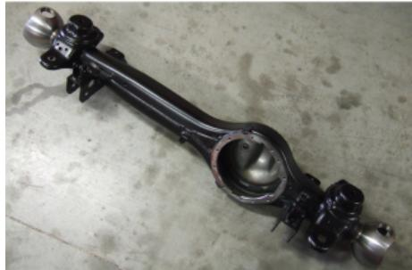
**CORPS PONT AVANT AVEC BLOCAGE POUR
