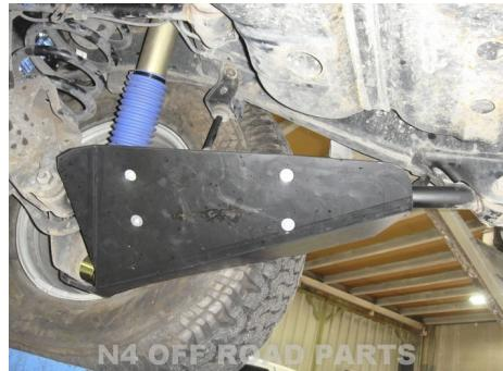
**N4 OFF ROAD PARTS****PROTECTIONS D'AMORTISSEURS N4 (PEHD 8MM)
