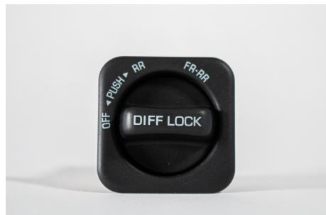
**COMMANDE/BOUTON BLOCAGE DE DIFFERENTIEL AVANT ET ARRIERE**
