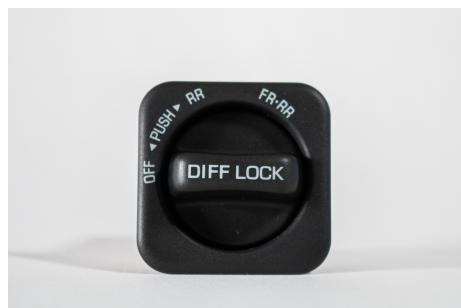
**COMMANDE/BOUTON BLOCAGE DE DIFFÉRENTIEL AVANT ET ARRIÈRE**
