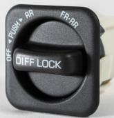
**COMMANDE/BOUTON BLOCAGE DE DIFFERENTIEL ARRIÈRE**
