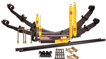
**KIT DE SUSPENSION LAMES PARABOLIQUES
