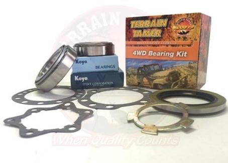
**KIT ROULEMENT DE ROUE AVANT OU ARRIÈRE
