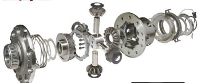
**ELocker®****BLOCAGE DE DIFFERENTIEL ELOCKER ARRIERE 100% ELECTRIQUE**
