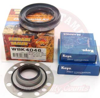
**KIT DE ROULEMENTS DE ROUES ARRIERE TERRAIN TAMER (POUR PONT AVEC AXE FLOTTANT & TAMBOURS DE FREIN)**
