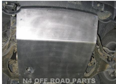
**N4 OFF ROAD PARTS****BLINDAGE AVANT 8MM N4 POUR NISSAN NAVARA D40 A PARTIR DE 2005 ET PATHFINDER**
