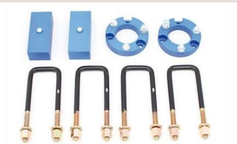
**KIT CALES DE REHAUSSE SUSPENSION SUPER PRO POUR NISSAN NAVARA D40 (2005-2014)**
