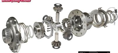
**ELocker****KIT BLOCAGE DE DIFFÉRENTIEL ELOCKER AVANT
