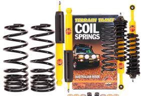
**KIT DE SUSPENSION TERRAIN TAMER COMBINÉ ASSEMBLÉ REHAUSSE +40/50MM POUR TOYOTA FJ CRUISER A PARTIR DE 2010**
