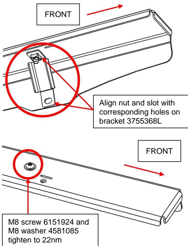
3.1) Take the stay bracket (561AQ067) and align M8 weld nut to underside of LH blade bracket (3755368L) round hole and lower slot with vertical slot at front of the bracket.
