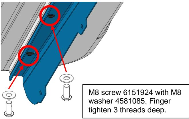
3.8) Slide the crosswise support brace (560PD063) with the open slot between the C-channel rail on the tent and blade bracket at the two inner M8 screw locations each side.
