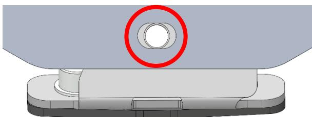
4.1) Confirm blade bracket holes are correctly aligned to vehicle.
