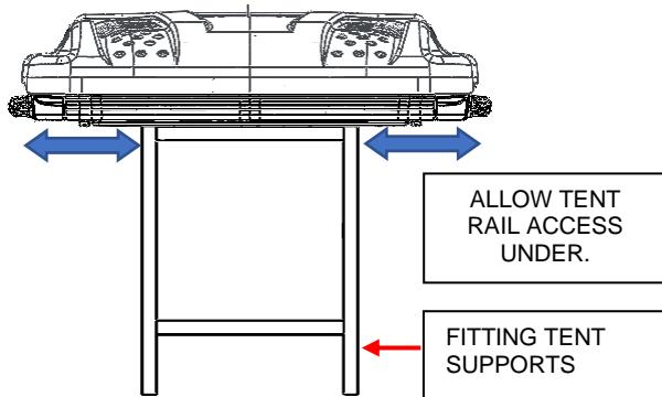
3.0) Place the tent on a clean flat surface. Provide protection to the bottom face of tent to avoid marking of surfaces. Make sure to have enough clearance at the bottom to reach the C channel rails on both sides, as attached to the underside of the tent.
