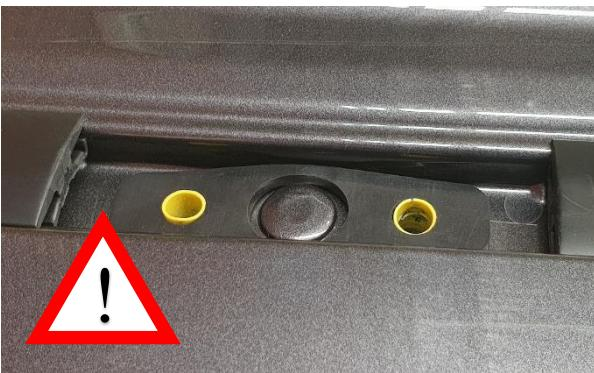
1.5) **IMPORTANT NOTE:** Anchors are sleeved with a thin plastic tube. When removing or installing brackets, be careful **NOT TO PUSH THE TUBES DOWN**. The anchors are connected to these tubes and will easily come loose with them.
