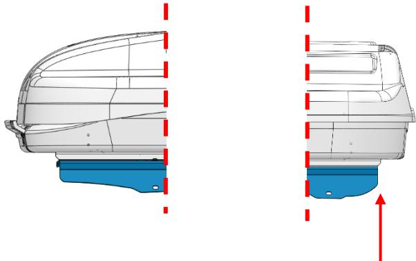
ALIGN BLADE BRACKETS TO REAR END OF C
