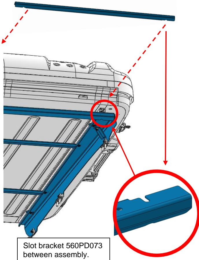
3.9) Slide the front crosswise support brace (560PD073) with the open slot between the C-channel rail on the tent and blade bracket at the front to engage around the bolts that retain the 561AQ003 nut plates at the front corners of the blade brackets.
