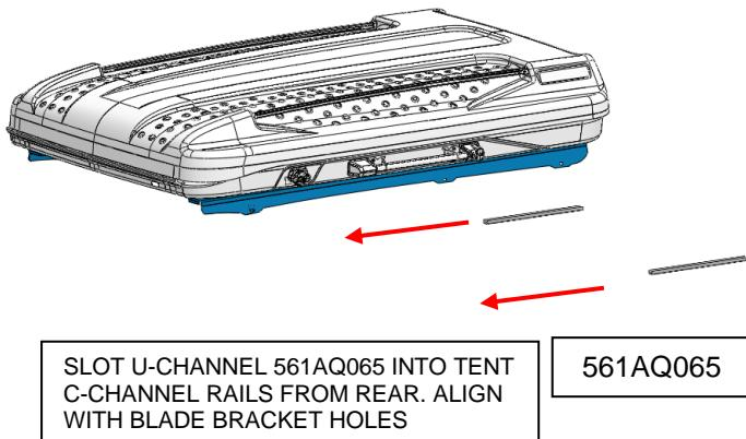
3.7) Slide two roof bar support brackets (561AQ065) into the rear of the C-Channel rails on the tent and align with corresponding holes in blade brackets.
