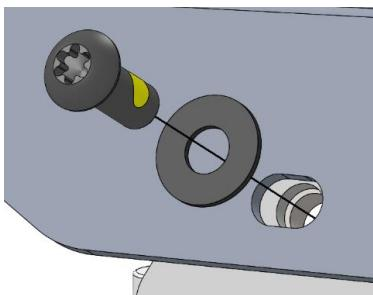
4.2) Use the M8 Button Head Torx screws and M8 Black washers supplied to secure the blade brackets to the roof mounting brackets. Tighten all screw to the specified torque.
