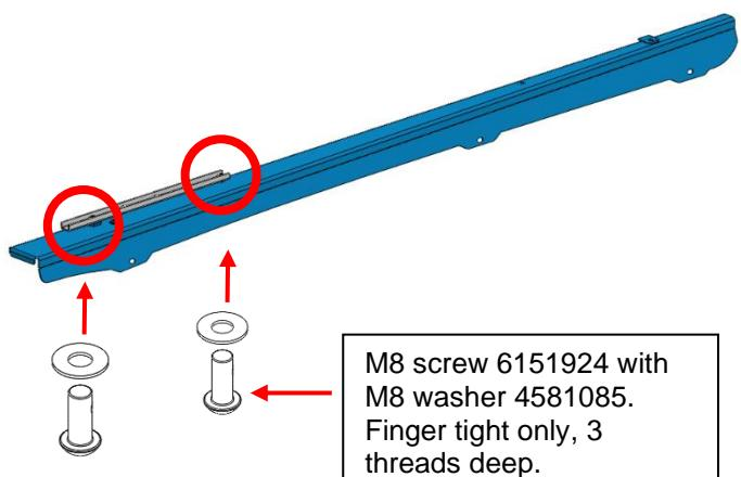
3.5) Align two M8 weld nuts of the roof bar support bracket (561AQ065) over the front two holes of the blade bracket (3755368L) with the longest end of the 561AQ065 bracket pointing forwards.
