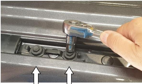
1.4) Remove all the brackets from the roof (except for anchor point 1b). Use 12mm socket for front and back factory roof rail brackets. Use 10mm socket for all other brackets. Discard plastic covers, rails, brackets & fasteners.
