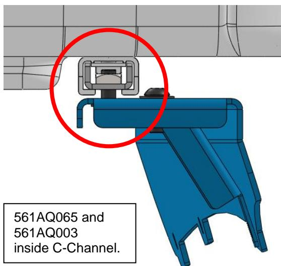
3.6) With the tent on supports, slide the roof bar support bracket (561AQ065) attached to the blade brackets into the C-Channel rails on the underside of the tent, including 561AQ003 as loosely fitted on the ends of the blade brackets.
