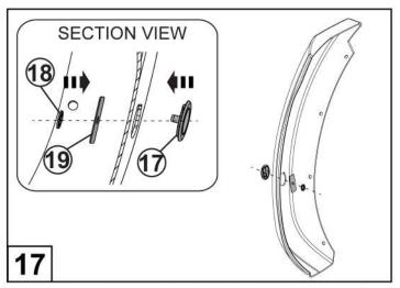
Fit the sensor cap and retaining strap to the fender flare, and secure with the starlock washer.
