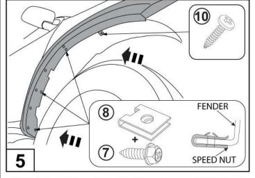
Hold the splash guard inwards and push the supplied (3x) 8.5 Speed Nuts onto the front guard into the 3 hole positions as shown. Fold the plastic Tab inwards over the fender and secure with one Phillips head screw.
