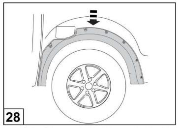
Fit the fender flare to the vehicle in the uppermost vertical position, before final fixings and tape application is completed as shown.
