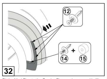
Fit the Mud Flap to the Fender Flare and secure with (3) 6mm plastic scrivets and one 10mm scrivet at the bottom, with one 5mm spacer.
