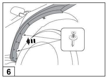
Reattach the wheel arch liner with two factory scrivets.
