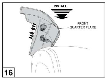
Hold fender flare assembly close to the bumper & fit Active park assist sensor to the escutcheon as per the Ford Workshop Manual (note the audible 'click' when the sensor is fully home). Skip to step 18.
