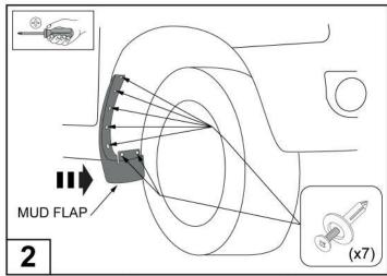
Remove the mud flaps by removing the (7) scrivets from inside the wheel arch as shown.
