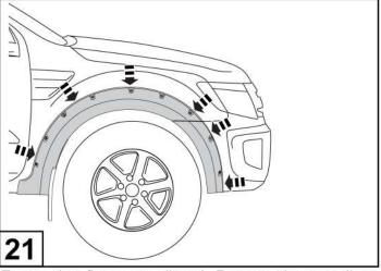
Ensure that flares are aligned. Remove the tape liner. Apply firm pressure on the flare to ensure the tape is contacting the vehicle surface around the full perimeter of the flares.
