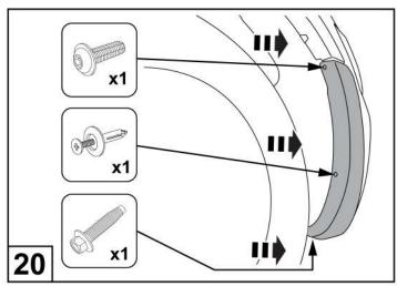
Secure the flare using previously removed screw and scrivet as shown.
