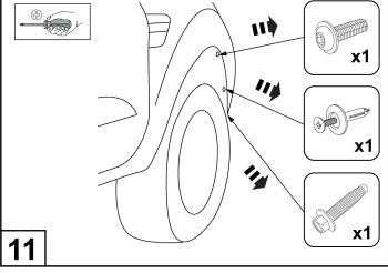
Remove and retain screw and scrivet from the wheel arch on the front bumper. Remove and retain the Hex head screw located under the bumper.
