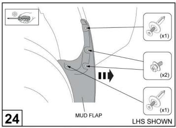
Remove the rear mud flaps by removing and retaining the (2) screws and (2) scrivets from inside the wheel arch as shown.
