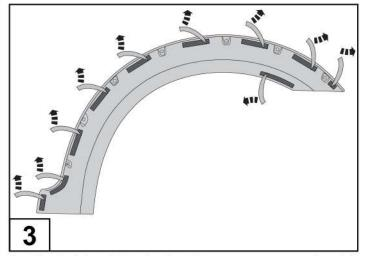
On the inside of the fender flare remove approximately 25mm of the protective liner from the double sided tape locations. Fold the liner over and secure with masking tape to the outside of the bumper flare.
