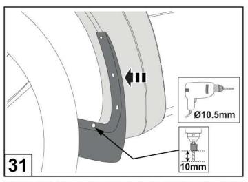
Fit the Mud Flap to the Fender Flare aligning with all the holes. Mark and drill a 10.5mm hole in the liner for the bottom scrivet as shown.
