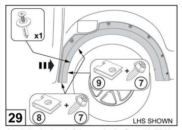
Attach the front part of the rear fender flare with (3) Hex head screws and Speed nuts as per front fender process. Reuse one factory plastic scrivet as shown.
