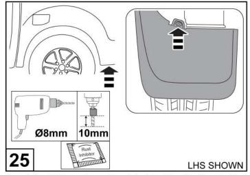
Carefully drill through centre of rivet holding the liner behind the rear mud flap, with a Ø8mm drill bit & and 10mm drill stop as shown. Carefully remove the reminder of the rivet using needle nose pliers. Apply rust inhibitor to the holes.
