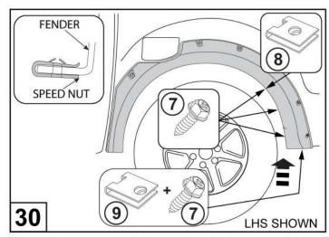
Attach the rear part of the rear fender flare with (3) Hex head screws and factory plastic nuts. Secure the rear lower part with one hex head screw and Speed nuts as shown.
