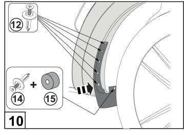
Fit the Mud Flaps to the Fender Flare and secure with (5) 6mm Plastic Scrivets. Secure the bottom part of the mud flap with one 10mm Plastic Scrivet and place the 5mm spacer behind the Mud Flap.
