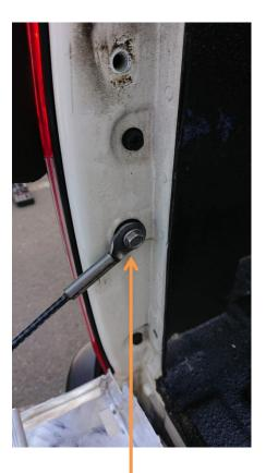
Do not discard this fastener, it is reused to mount the filler kit
