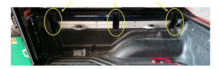
**NB!** The Canopy Camper must rest solely on the mounting brackets and no load is allowed on the load bin. Once this is completed, the Canopy Camper has been installed successfully.
