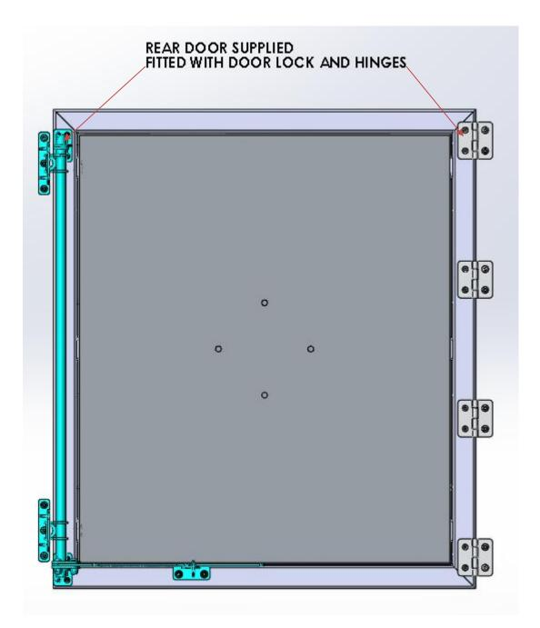
Attach hinges and lock to camper frame.
