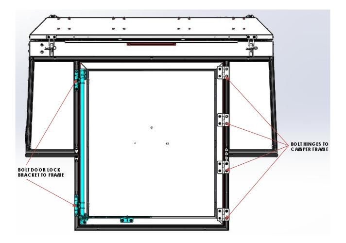
Fitting of front filler panels to base unit.
