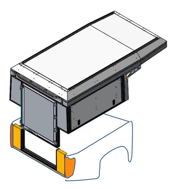
1. Connect rear filler panel assembly and base unit as shown.
