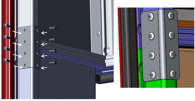
Fit rear door rebate with Ø4.8 x15 sealed countersink rivets as shown.
