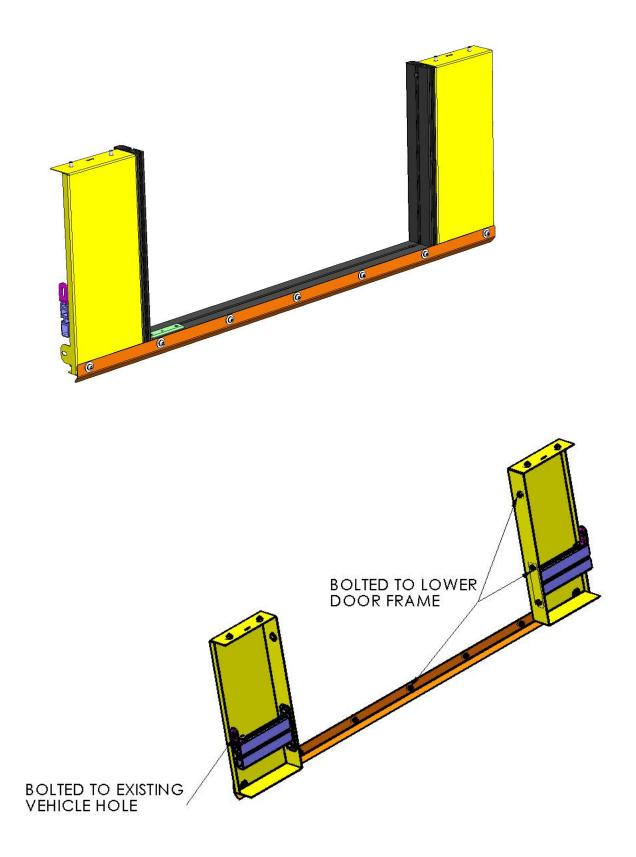
Fit lower door frame to filler panel assembly as shown.
