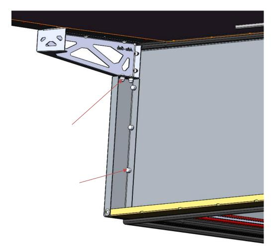
Rivet bottom filler panel on to bottom frame member using supplied Ø4.8x15 sealed rivets
