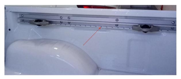
2.1 Fit 3 off mounting bracket set on either side of load bin to the pre fitted rail as shown above. Insert nut plate of bracket set into rail and bolt the bracket onto it.
