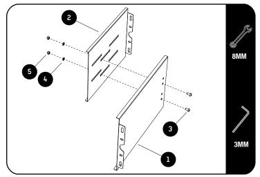
Slide the Slotted Divider Plate B (Item 2) into the Solid Divider Plate A (Items 1). Adjust the two plates to the approximate width of the Drawer and loosely fasten the two plates together using two of the M5 x 10 Button Head Bolts, two M5 x 10 x 1SS Flat Washers and two M5 Nyloc Nuts (Items 3, 4 & 5). The Flat Washer and Nyloc Nut go on the side of the Slotted Plate.
