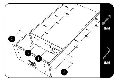
Depending on the drawer you have, you will be mounting to either the two outer holes or the inner holes on the side of the Drawer as shown in Step 2.2 and Step 2.3.
