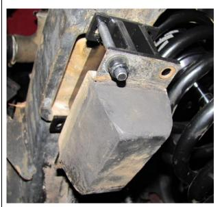
Install the supplied bump stop bracket between the bump stop and the chassis with the new supplied fasteners as shown in the pictures.
