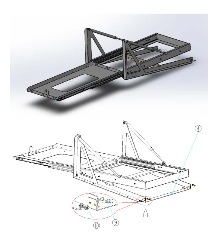
**Step 3:** Using the M6x20mm screws/M6 washers and tee nuts to install slide into vehicle.
