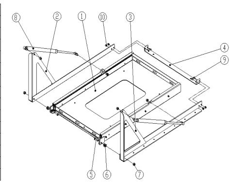
**Step 1:** Using the M8 bolts and nylon washer to install the left and right gas struts frame.
