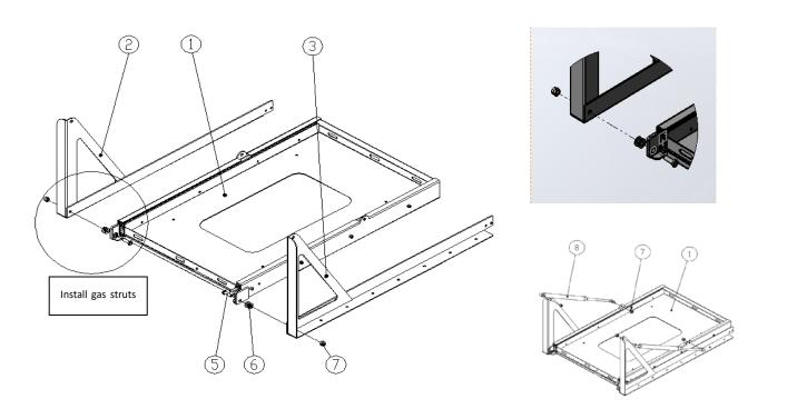
**Step 2:** Lift the body frame up to install the rear cross rib by using M6x12 bolts.
