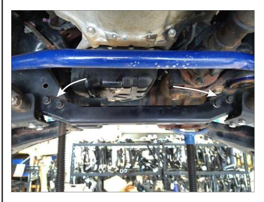
Bolt up new diff-drop bracket using supplied M12 x 75mm bolts (x4)
