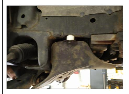
• Use the supplied 2 smaller nylon spacers for both sides of bash plate.
