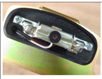
9. Secure light to bracket using M5 pan head screws and flange nuts.
