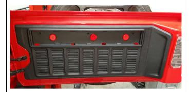
1. As the number plate is normally mounted on the bumper bar, a number plate relocation bracket is required.
