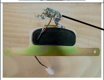
8. Fit loom to light as shown. Note position of white and brown wires.
