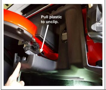
4. Remove the plastic screw that retains the tail light. Then unclip the rear R/H panel to expose the seat belt mechanism and the wiring loom for the taillights.
