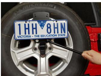
14. Fit the plate onto the bolt shank as shown. Then use the wheel brace to tighten the bolts up securing the plate. ..
