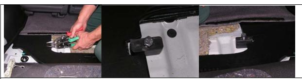
**2.12/-** Loosely bolt front mount rail down using 10mm X 60mm bolts, spring washers and 75mm X 40mm flat oblong washer and into front exposed holes.
