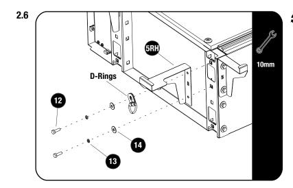
Assemble the Rear Side Wings (Item 4) together with D-Rings (supplied with SSDR011) to the rear left and right side of the drawer, using M6 x 20 Button Head Bolts, M6 SS Spring Washers and M6 x 19 x 1 SS Flat Washers (Items 12, 13 & 14) as shown.
