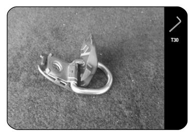
Loosen and remove the two front and two rear tie-down points in the back of the vehicle.
