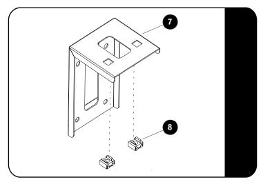
Fit the two M6 Cage Nuts (Item 8) to the Back Support (Item 7) as shown.
