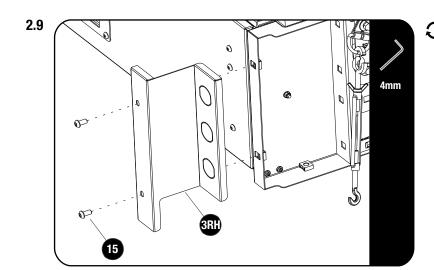
Secure the Front Faces (Item 3LH & 3RH) to the Drawer using M6 x 16 Button Head Bolts (Item 15) as shown.
