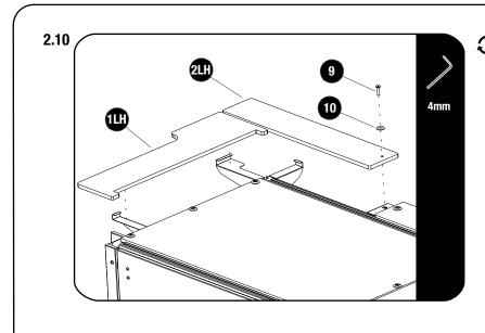
Fit the Side Decks and Rear Decks (Items 1 & 2) to the Drawer by placing them into the C-Clips and pushing downward. Secure the middle of the Rear Decks using M6 x 30 Countersink Screws and M6 Finishing Washers (Items 9 & 10) as shown.
