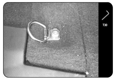
Refit the two rear tie-down points so that the D-rings face outward toward the side.
