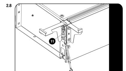
Secure the Drawer to the vehicle's front mounting points using two Turnbuckles and two 37mm Laser Cut Carabiners (Item 11) as shown.
