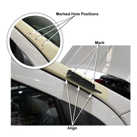
Drill a pilot hole at each of the three marked hole positions.
