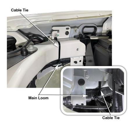
Cable tie the washer hose and/or loom along the path shown using the remaining cable ties (item's 19 & 20) where required, so they do not come into contact with the air entry hose (item 10) when installed.
