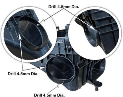
Install the air cleaner inlet adaptor (item 11) into new air cleaner base inlet.
