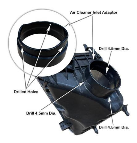
Remove air cleaner inlet adaptor (Item 11) from air cleaner base and clean both mating surfaces.
