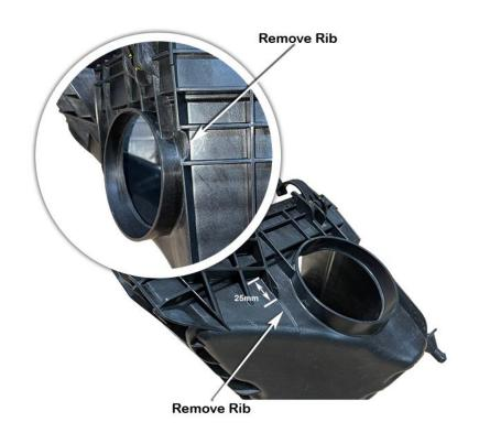
Measure and mark the three hole positions around the new air cleaner base inlet hole as shown.
