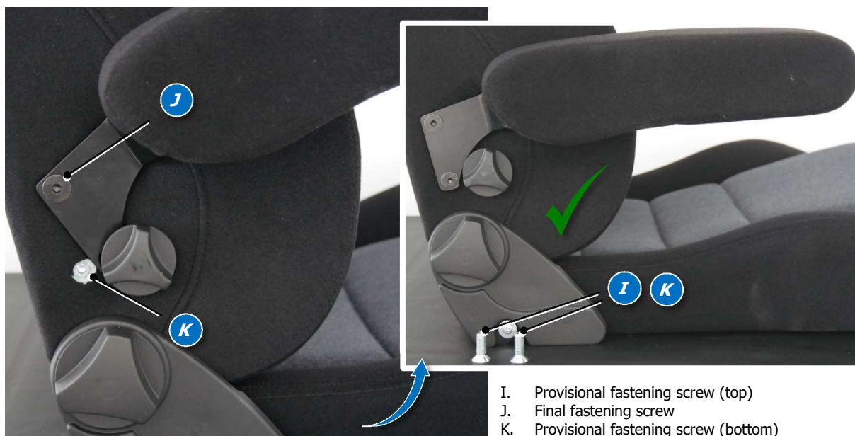
Fig. 8 Mounting the armrests (option) - screw in and tighten the final fastening screws
