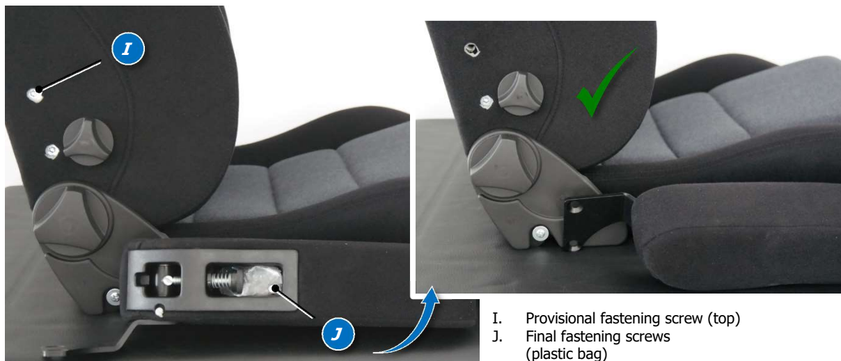
Fig. 7 Mounting the armrests (option) - remove provisional fastening screw (top)
