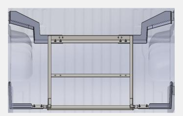
USE THE TAPE MEASURE TO MAKE SURE THE FRAME IS CENTRAL. TIGHTEN ALL FIXINGS.
