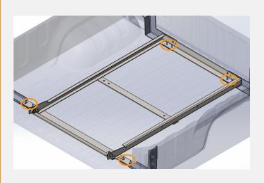
PLACE THE BOTTOM FRAME IN THE BED, LOCATING ON THE PROTRUDING BOLTS IN THE BRACKETS.
