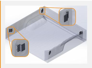
USE THE BOLTS JUST REMOVED TO SECURE THE Z BRACKETS TO THE BED IN THE POSITIONS SHOWN.
