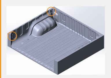
LOCATE THE MANUFACTURERS 4 TIE DOWN POINTS AND REMOVE ANY HOOKS ATTACHED (2 AT THE BULKHEAD, 2 AT THE TAILGATE).
