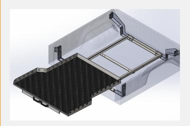
REVERSE STEP 1.5 TO ATTACH THE TOP FRAME TO THE BASE. (COMPRESS THE BUTTON ON THE HANDLE, TILT, DROP IN BETWEEN THE TRACKS, GENTLY LOWER AND PUSH BACK).
