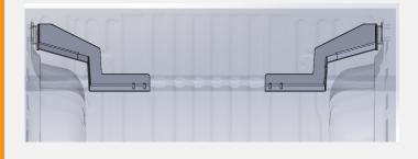
USE THE M8 X 20 BOLTS TO LOOSELY ATTACH THE BULKHEAD BRACKETS TO THE Z BRACKETS.
