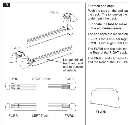
Push the tabs on the end cap through the slots on top of the track. The tongue on the back of the end cap must lie
