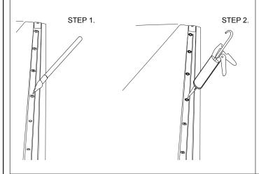
1:Remove the backing tape from the ButylPatches.
