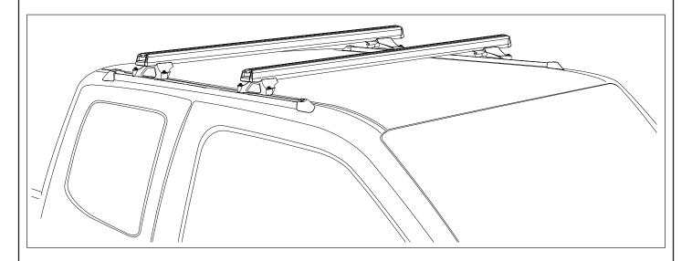
**SPECIAL NOTE:** Assistance by a second person is recommended to put downward pressure on the track while the holes are marked out and drilled.
