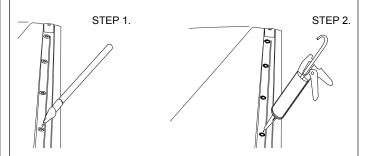
1:Remove the backing tape from the ButylPatches.
