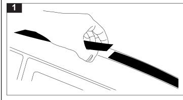
Unclip to remove the bolt cover plates towards each end of the roof gutter trim. Lift and remove the long middle section trim from the roof starting at the front of the vehicle. The shorter trim at each end can be left in place.
