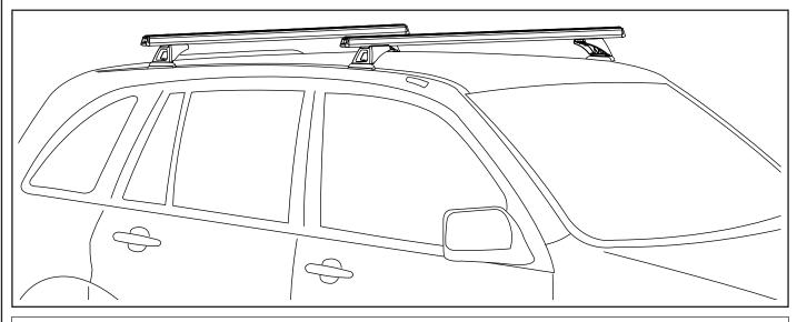
Care Instruction: Thoroughly clean under the roof channel trim when removed prior to installation.
