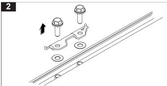
Using a 10mm socket wrench remove the two bolts and brackets at each end of the roof channel. Do not remove the rubber coated washer on these bolts. **Keep the bolts and washers as they will be used to fasten the track to the roof.**
