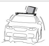
WARNING: Cabin and canopy move independently on utility vehicles. Rigidly fix items to either the cabin roofracks or the canopy roofracks, as fixing on both simulaenously will cause damage.
