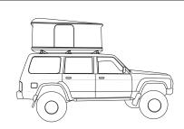
When vehicle is driven off sealed roads, the maximum roof rack load rating should be divided by 1.5. Do not forget to subtract 5kg from your maximum carrying capacity due to the weight of the crossbars and legs.
