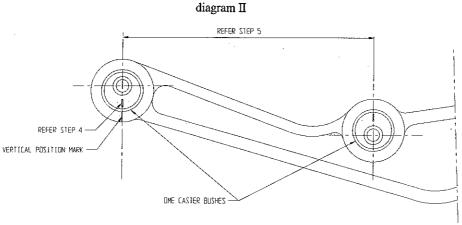
5. Install the second bush by positioning the bush pin centre at the same centre spacing previously taken from the original bush centres in 2. above.
