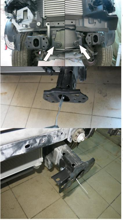
14. Remove plastic dusters from left and right sides of the vehicle.
