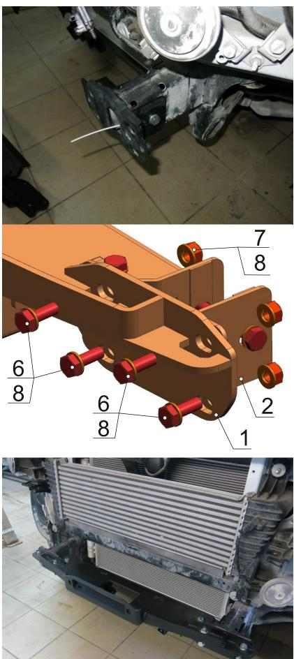
17. From outside of the chassis, mount outer bracket (2) from both left and right side. Fix them with bolts M10x30 (6), washers (8) to insert nuts (5).
