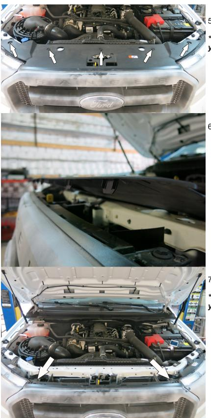
5. Remove 4 screws out of radiator grill.
