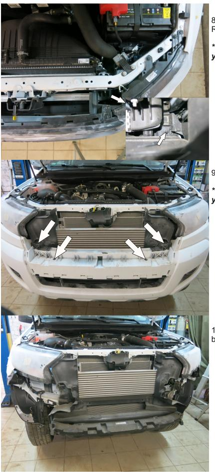
8. Remove 2 screws out of radiator grill. Remove radiator grill.
