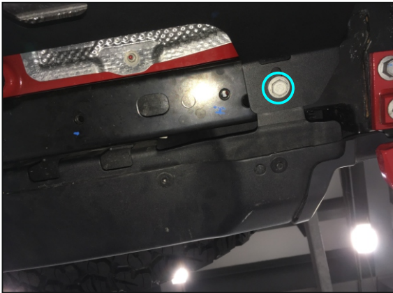
3. Unscrew bumper's fitting bottom bolts.
