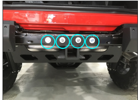
14. Install tow bar square (pos.5) using bolts M12x120 (pos.F), washer 12 (pos.J) and nuts M12 (pos.N). Torque hardware to * M12 - 77 Nm (56.8 lb/ft) .
