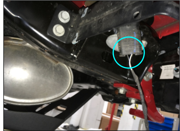
2. Disconnect license plate lights on the left side of the vehicle.
