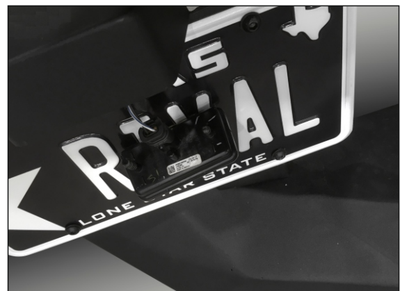
18. Connect wiring of the license plate bracket lights through the license plate hole.
