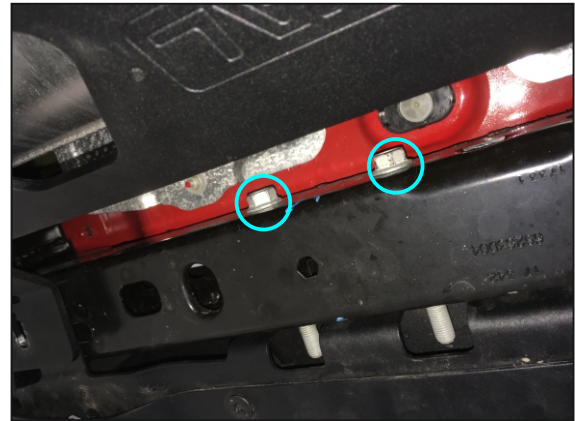
4. Unscrew bumper's 2 fitting bolts from the rear beam.
