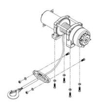
make sure the motor, drum and gearbox housing are aligned correctly.
