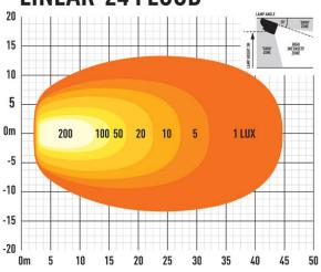
Generated from BSI lamp photometric test data: on road measurement data
