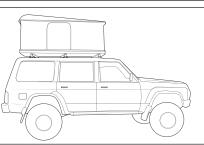
When these roof racks are to be used on a vehicle that is driven off sealed roads the maximum load rating must be divided by 1.5.
