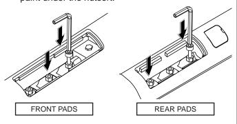
Assemble the spring and flat washers onto the security socket screws. Insert the screws into the pad mounting holes and using the allen key carefully tighten. Recommended tightening torque 4N/m. **DO NOT OVERTIGHTEN.** Repeat this process for each pad.
