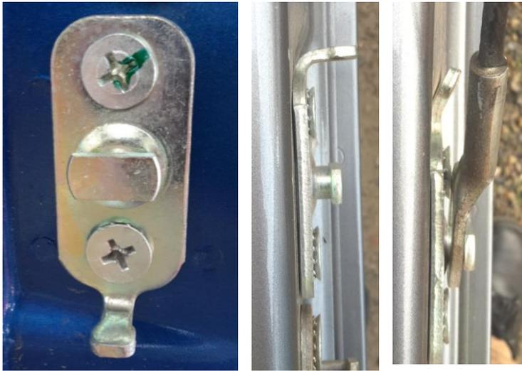
**1.3)** If the tailgate is fitted with cables, the tailgate retainer will have a bent tang on the lower side of it. Remove the retainer and straighten the tang so that it follows the line of the panelwork.
