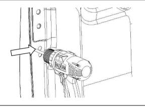
1.7) Drill marked hole out to 8.5mm. De-burr and paint or when complete.
