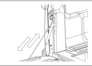
2.3) When complete open and close the tailgate to ensure correct operation. Make sure there is no binding, cables protruding or contact of struts to the vehicle tailgate or body of the vehicle.
