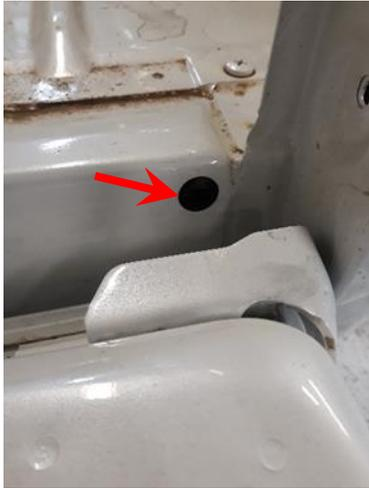
1.1 Open the tailgate. Remove and discard the rubber bung (if fitted) on the body of the tub near the RH Hinge.
