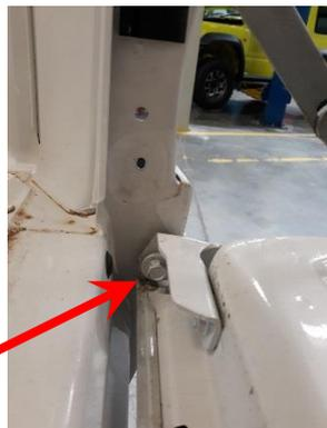
1.3 Remove the hinge bolt from the RHS of the tailgate and discard.
