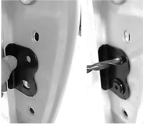
2.8 Remove the Bracket and reassemble using the 3195150 Plate on the inside of the Tail Light cavity to sandwich the panel.
