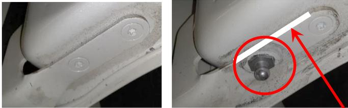
4.2 On the tailgate, remove the countersunk hinge screw nearest where the tailgate mounts to the vehicle and replace with the 6151908 Countersunk Ball Stud.
