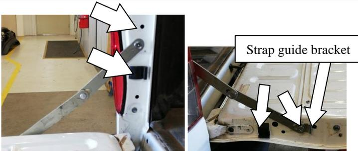
4.1 Ensure RH side strap is holding the tailgate and similar to RH side follow steps, 2.1 to 2.4 to remove the OEM straps on LH side.
