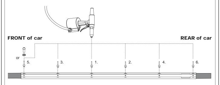
11 Insert both End Caps (Item 2,3) into the FRONT and REAR of BOTH tracks as shown.
