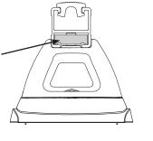
Adjust cross bar overhang to be equal both sides. Once adjusted tighten M10 crossbar bolts to 8-9 Nm (6-7lb/ft). Then fasten M6 security screws to 4-5 Nm (3-4lbf/t).
