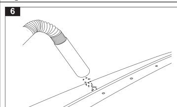
Use a vacuum to remove swarf to eliminate scratching. Wipe clean the installation area of the roof.
