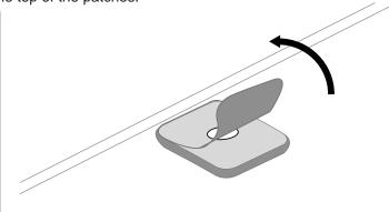
Peel the white backing strip off the track foam tape.
