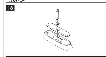
Pad cover plates are provided for when crossbars are removed.
