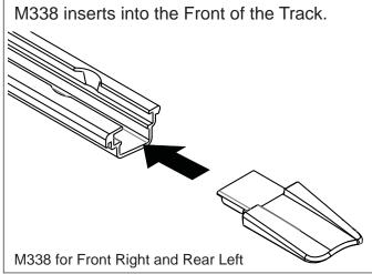
Side View: The end caps will slip into the channel on the installed track. The end caps may be gently flexed to achieve this.
