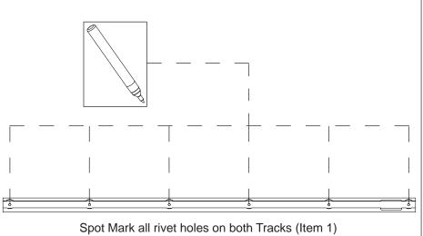
All 6 holes can now be drilled through. A drill stop must be used to prevent drilling through the hood lining on the inside. **Make sure that when drilling you hold the drill perpendicular to the roof angle.** The roof skin is approx. 2-3mm thick.
