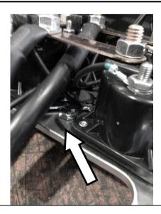
Undo 2 X supplied M6 nuts from underside of control box. To do so, top of M6 bolts located on the inner side of the box will need to be held in place.
