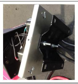
Attach control box to control box bracket using fasteners removed from control box in earlier step, so that the top face of the bracket is flush with the bottom surface of the control box.
