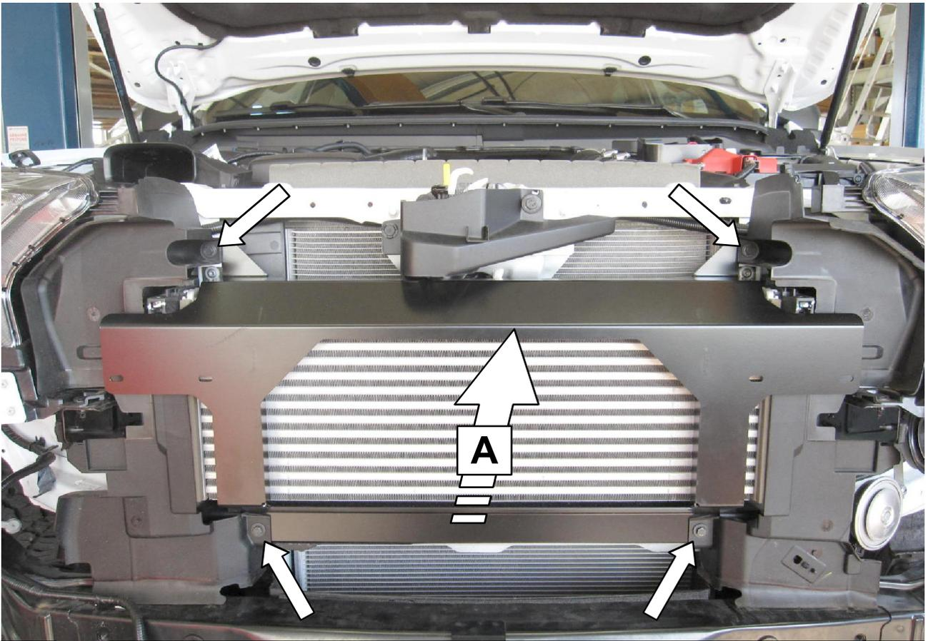
**6** Original Schrauben verwenden! / Use the original screws!
