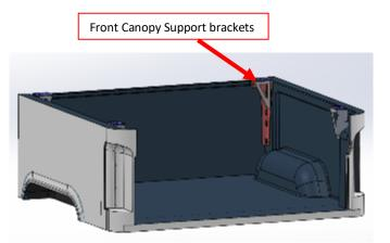
Figure 8: Front Canopy Support Bracket Position
