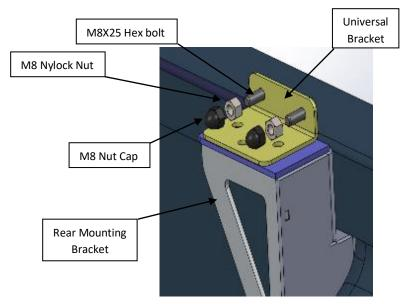
Figure 19: Rear Universal to Canopy Mounting assembly
