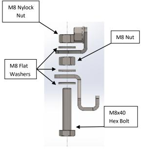
Figure 13: Centre Bracket Mounting Assembly
