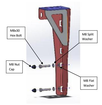
Figure 10: Front Bracket Mounting Assembly
