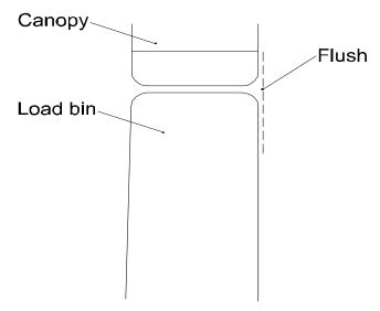
Figure 16: Canopy and Load Bin Alignment
