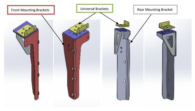
Figure 1: Front Support Canopy Brackets
