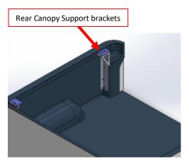
Figure 7: Rear Canopy Support Bracket Position
