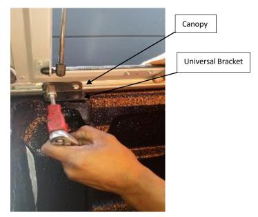
Figure 21: Tightening Universal bracket to Canopy
