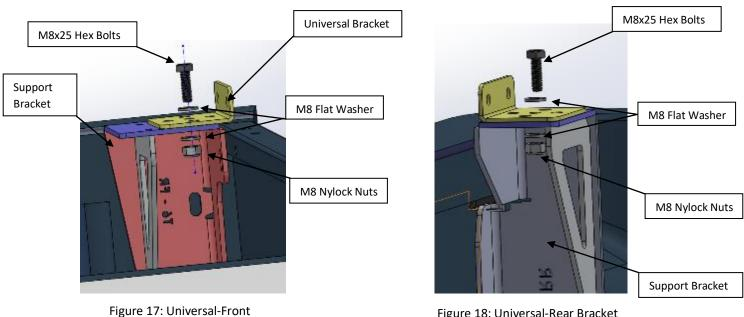
Figure 17: Universal-Front Bracket Mounting Assembly
