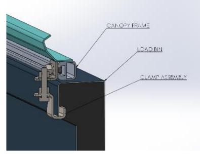
Figure 15: Section View of Clamping Method
