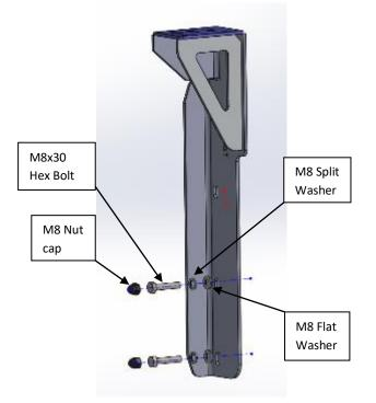
Figure 9: Rear Bracket Mounting Assembly
