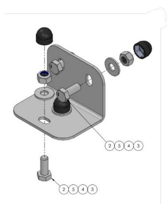
**The Universal Load Bar Mounting Bracket** to be fitted to the sides of the Tent for extra support and stability as shown on page 2 and page 8
