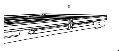
(G) Once the Rack has been mounted to the vehicle, open the Latch by pushing on the Latch Release and slide the Table into position. A small padlock can be used through the hole in the Latch Release should you wish to lock the table.
