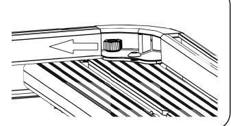
(F) Place the Latch (Item 9) onto the Rack, lining up the mounting hole in the Latch with the Nyloc Nut inserted in Step 2E. Secure the Latch in position using the M8 x 20 Button Head Bolt and M8 Flat Washer (Items 7 & 8).
