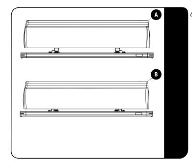
Hard shell tents may need additional support. If you are using these brackets with hard shell tents, such as James Baroud or Autohome, and you are unable to position the tent to rest directly on the rack side profiles (A), use TBMK009 – Hard Shell Tent Support Channels - by Front Runner (B) sold seperatly.
