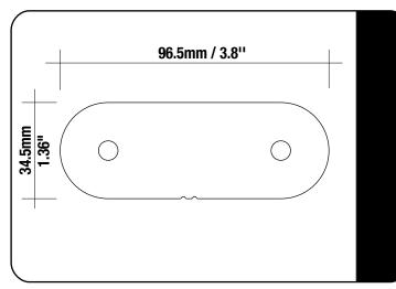
The Tent Channel Nut Plate included were designed for the Front Runner Tent but will also work with other popular tents. Check your mounting channel measurements for the appropriate size.
