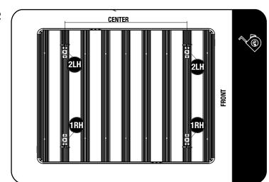
Measure the distance between the center points of the Rack Mount Brackets. You will need this measurement for fitting the Latch Bracket assembly to the tent channel in Step 2.5.
