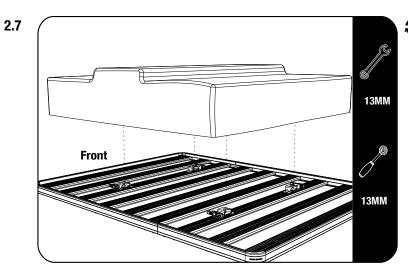
Flip the tent over and lower it onto the rack making sure the Bobbins align with the rack mount brackets.
