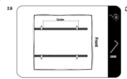
Measure the distance between the centers of Channel Feet to make sure it matches the position of the Rack Mount Brackets installed in Step 2.2.
