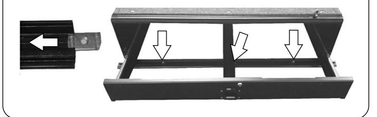
(E) Looking at the rear of the Drawer System, remove the bolts as indicated by the arrows. Keep the bolts and washers safe as they will be used at a later stage.
