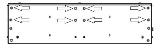
(F) Using six M6 x 20 Hex Hex Bolts, six M6 Spring Washers and six M6 x 19 Flat Washers removed in Step 2E, secure the Rear Support (Item 23) to the back of the Drawer System as shown.
