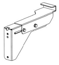
(**B**) Using Step 2A as a guide, loosely assemble the Corner Wing Sets (Items 24, 25, 26) as shown.
