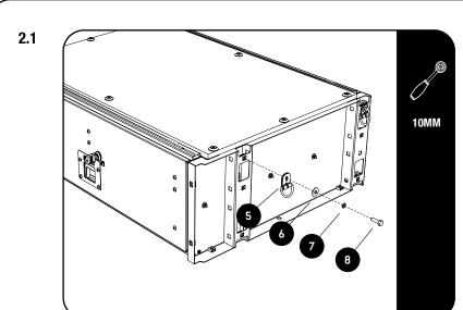
Secure the 4 D-Rings (item 5) on both sides of the drawer using the fasteners shown.
