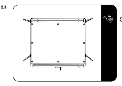
Place the drawer in the vehicle and position as desired. Making sure the turnbuckles are pulling outward to prevent the drawer from moving after it has been secured.
