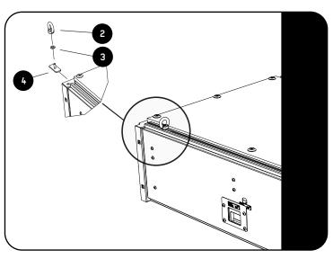
Assemble the eye-nuts (item 2) with a M6 nylon washer (item 3) and a stud plate (item 4) and slide them into place.
