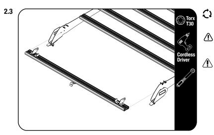
Secure assembly 2.2 to the front two top holes on the foot rails using the fasteners supplied with KSFR006.
