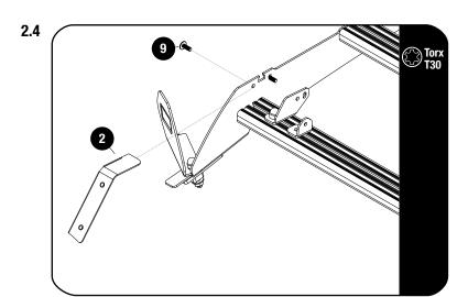
Swing over the Dimple plate to allow access to tighten the bolts.
