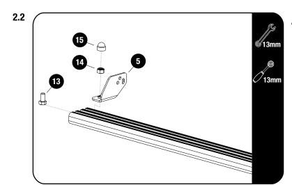
Fit the Light Bar Bracket 01 LH / RH (Item 5 & 6) for for the 40" Light Bar, using M8 x 16 Hex Bolt & M8 Nyloc Nut (Items 13 & 14). Fit the light bar and center it on the slat before fully tightening the brackets.
