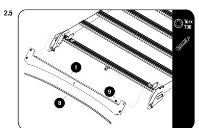
Fit the Wind Fairing Rubber (Item 8) to the Light Bar Wind Fairing (Item`1). Using the notched section as a guide, trim if needed.
