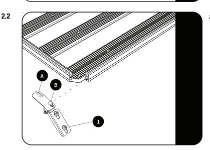
Slide 4 loosely assembled Wind Fairing Adjustable Brackets (Item 1) into the bottom T Slot as shown. Use either Slot A or B as shown in Figure 2.2.
